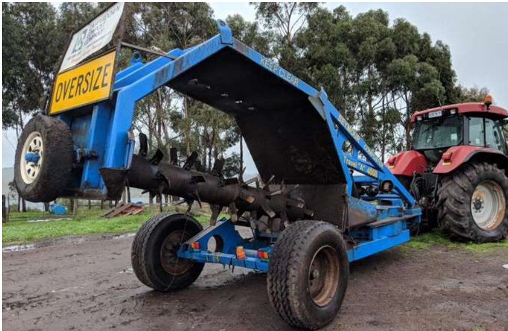
Figure 11. Compost turner designed to rotate for easier towing on public roadways.
