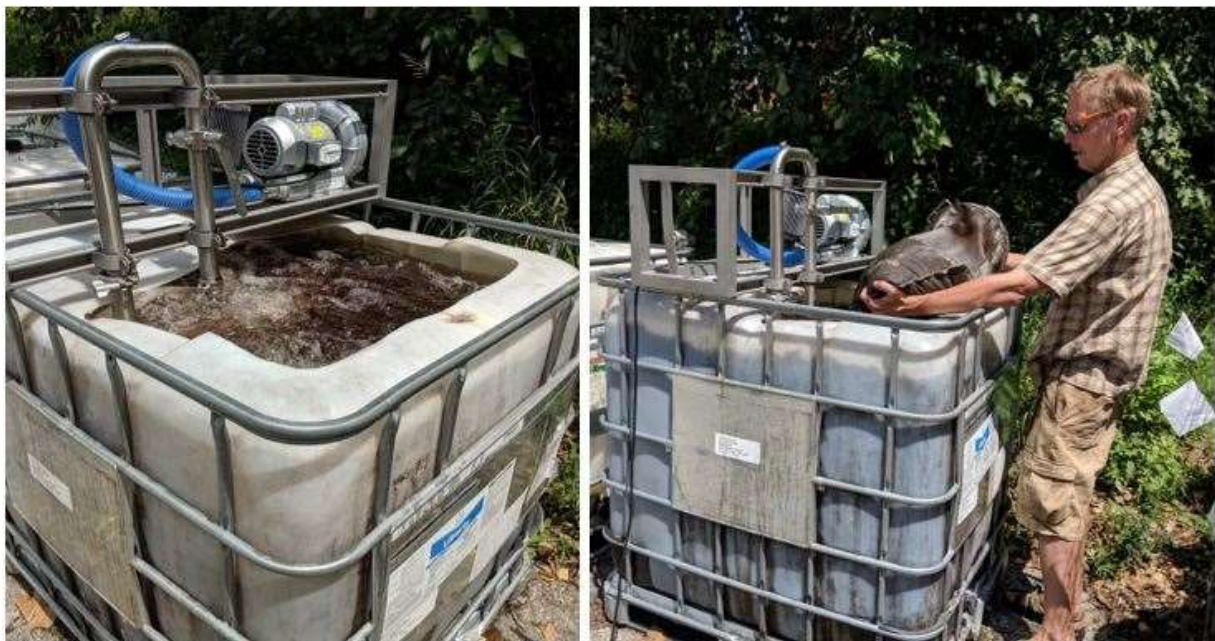
Figure 12. Michael Luebbers making compost extract with a GeoTea™ compost tea brewer for field application near Waverly, Iowa.
