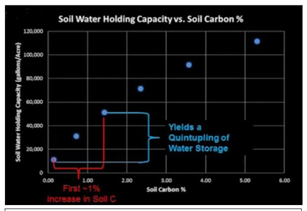
**Fig. 74.** Soil water holding capacity of soils with increased carbon content from the UTube presentation *'The BEAM Approach'* by Dr D Johnson, with many thanks to the author (Johnson, 2017).
