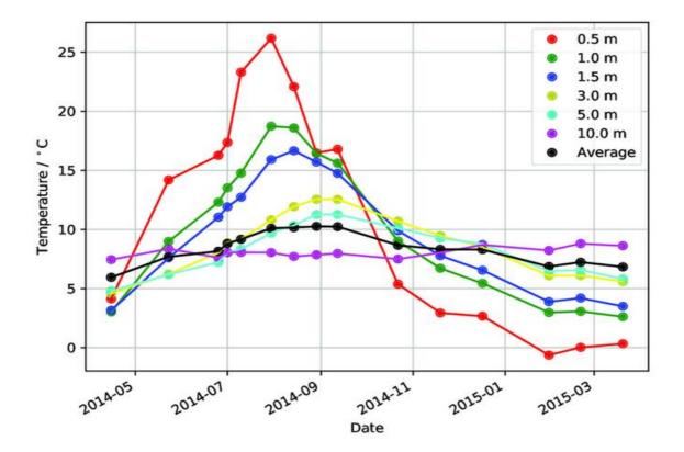
Soil temperatures measured at different depths (0.5 m, 1.0 m, ..., 10 m) and the weighted average temperature of the whole 10 m deep layer.
