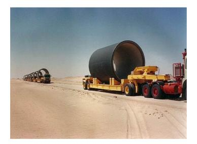
Fig, 26. Transportation of pipe segments in the 1980s for the Great Manmade River in the Desert, Libya. Sahara This network of pipes supplies water from the Nubian Sandstone Aquifer System, a fossil aquifer in region. The Great Manmade River is the world's largest irrigation project with abstraction estimated at 2.4 km<sup>3</sup> per year. With many thanks to Jaap Berk.
