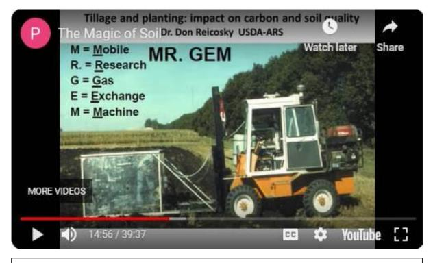
**Fig. 76.** *'Magic of Soil'* Philip Gregory, equipment used by Dr Don Reicosky for measure carbon dioxide loss following tillage. With many thanks to the Author. (Gregory, 2017)
